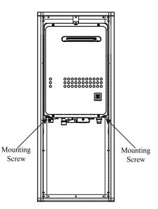
Figure 4: Location of lower mounting brackets.
