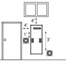
Figure 1: Discharge Vent Clearances.
